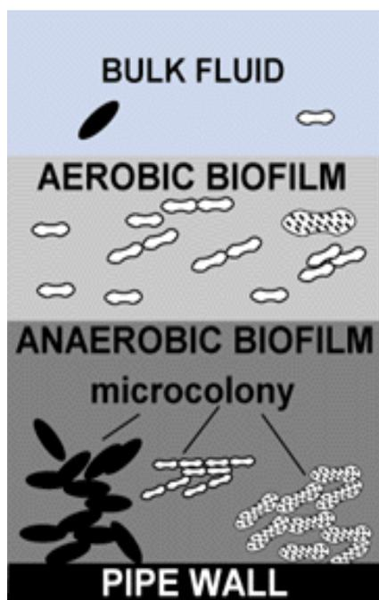
The biofilm begins when an iron pipe is in contact with water for example. The biocorrosion appears because bacteria alter the environment locally and because a biofilm is heterogenic: there are aerobes and anaerobes bacteria and most of time aerobes bacteria are near the fluid and anaerobes bacteria are closed to the metal. Moreover, the biofilm has different thickness.
